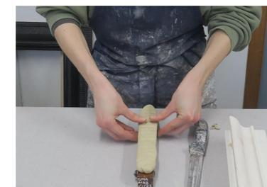
Pressing the composition onto the mould
